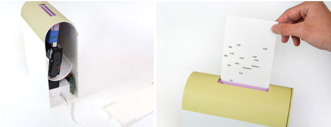
Figure 11: Left: Data Bakery includes a small WiFi connected printer that prints the recipe amounts for a cookie recipe (right).
