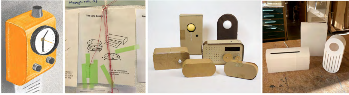
Figure 2: From left to right: Early sketches of Broadcast and Data Bakery; Form and function cardboard prototyping for Broadcast; 3D printed cases
